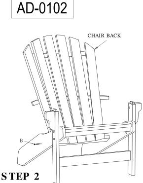
Tenons on the Back Assembly will fit into mortise (pocket) in Base Assembly. Attach with Screws (B) as shown).
