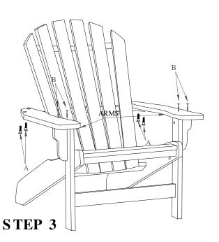
Attach Arms to front Legs from the top using screws (B). Bolt Arm Assemblies to Back Assembly using Bolts (A) as shown.
